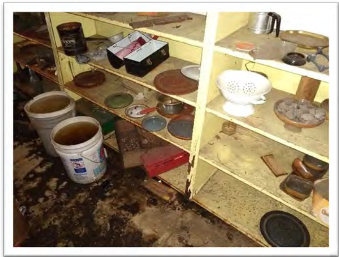
Sample 20-045A.L8, Yellow Paint, 68,000 ppm Lead
