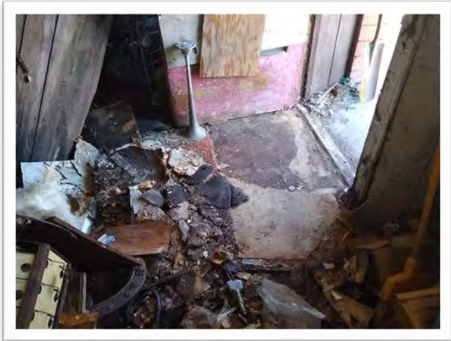
Sample 20-045A.1, Vinyl Floor, 20% Asbestos
