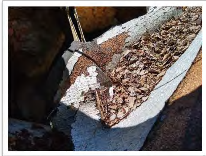
Sample 20-045A.19, Roof Coating, 2% Asbestos
