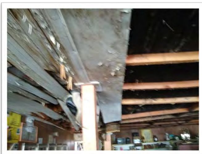
Sample 20-045A.L5, White Paint, 550 ppm Lead
