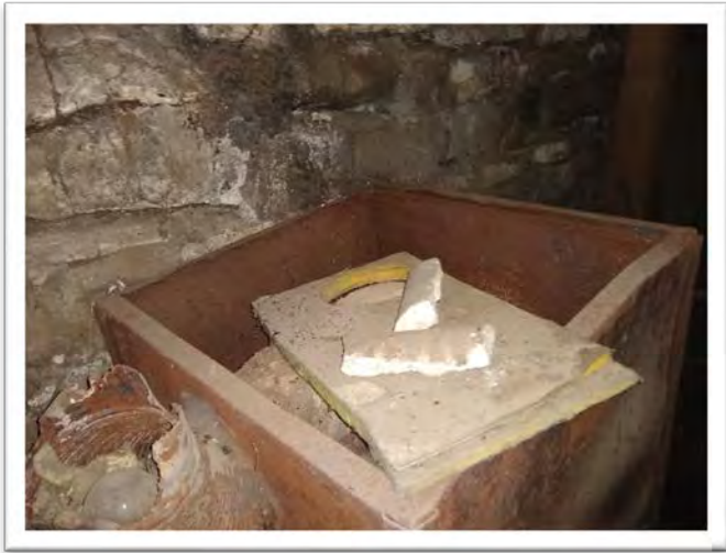
Samples 20-045A.43, Pipe Insulation, Non-ACM
