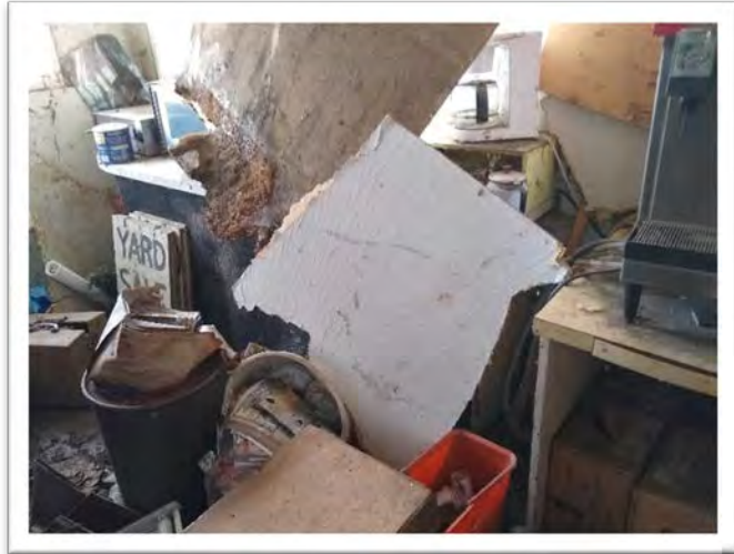
Sample 20-045A.17, Ceiling Panel, Non-ACM
